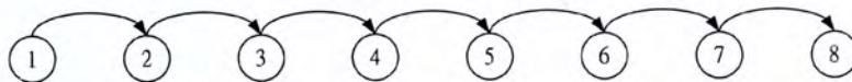
Figure 2.1. UDP traffic flow with node 1 as the source and node 8 as the destination in an 8-node multi-hop traffic flow
