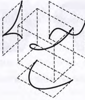
Figure 5.1: 2D Projections unable to fully describe the 3D information of the space curve.
