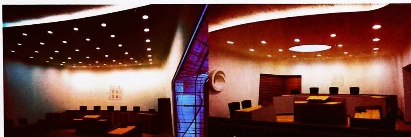
Light is admitted through an elliptical shaft directly above the speaker's podium of one of the courtrooms
