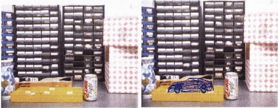
Figure 1.1: An example of augmented reality. A synthetic car, which is drawn by wire-frames, has been put on top of the yellow box in the real scene.
