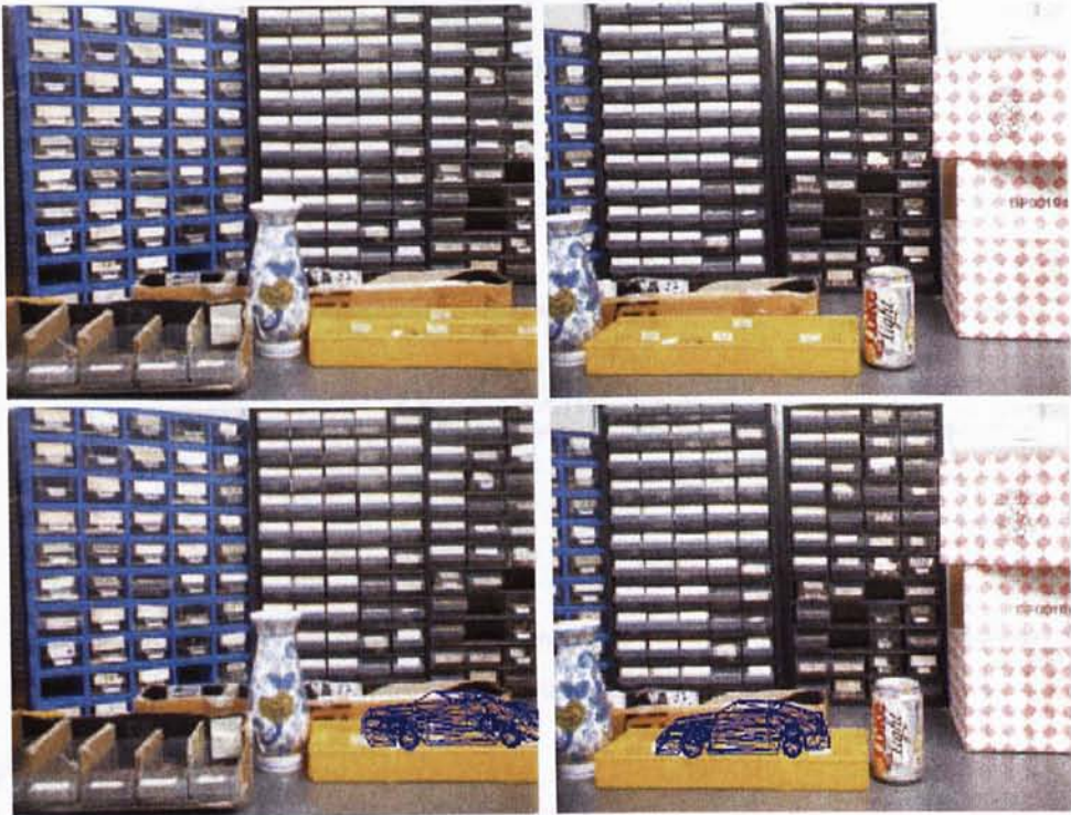
Figure 5.5: Results of augmenting an artificial object into the first test image sequence using the proposed IMM-based approach. First row: The first and the last image of the first test sequence. Second row: A synthetic car, which is drawn by wire-frames, was augmented into the scene. The original and the resulting augmented reality video can be downloaded at http://www.cse.cuhk.edu.hk/~vision/demo/
