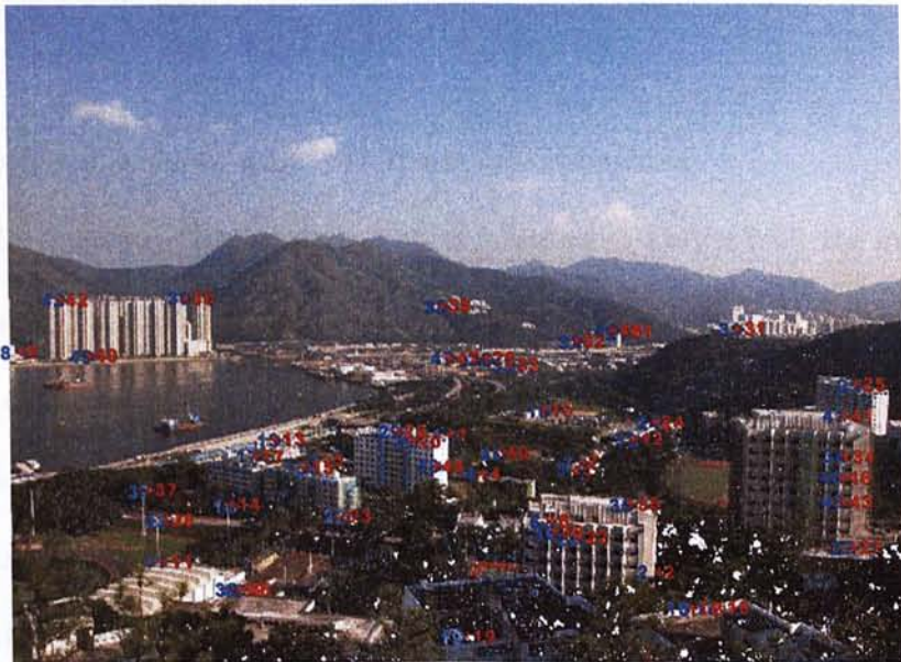
Figure 12: Image 2 of the distant scene, with the manually picked (true) correspondences of the 49 feature points marked as red “crosses”, and the reprojection positions (from Image 1) of the correspondence-free algorithm marked as blue “crosses”.
