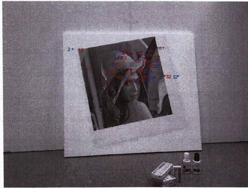
Figure 17: Image 2 of the scene, with the manually picked (true) correspondences of the 40 feature points marked as red “crosses”, and the projected positions (from Image 1) of the correspondence-free algorithm marked as blue “crosses”. Considerable reprojection error is shown in this figure.
