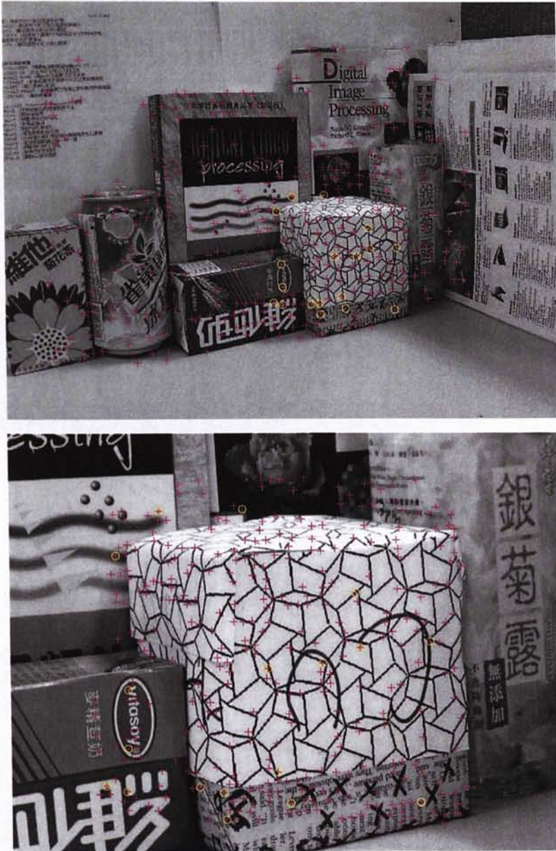
Figure 4.18: The result of the rematching algorithm for the “Box” scene. (Upper) The coarse image, (Lower) the fine image. The plus signs are the points tracked by the KLT tracker and the points circled by yellow circles are the rematched points.
