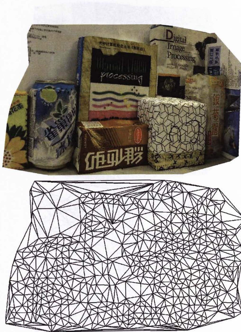
Figure 4.19: The 3D coarse model for the “Box” scene. (Upper) The texture-mapped 3D model and (Lower) the wire-frame 3D model.
