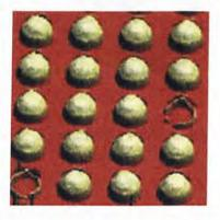
Figure 2.11: 3D Z-topography of bare die showing a bump defect
