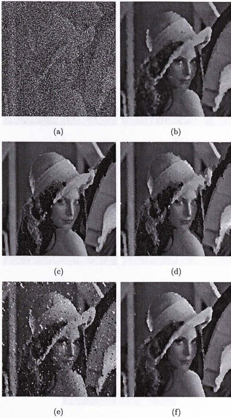
Figure 3: Restoration results of different filters: (a) Corrupted Lena image with 70% salt-and-pepper noise (6.7 dB), (b) MED filter (23.2 dB), (c) PSM filter (19.5 dB), (d) MSM filter (19.0 dB), (e) DDBSM filter (17.5 dB), (f) NASM filter (21.8 dB)
