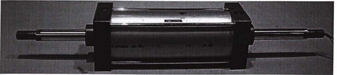
Figure 4.18: Assembled MR damper I.
