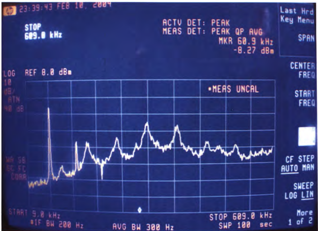
Fig. 5.4 Output Spectrum of Single Channel of Complex Modulator
