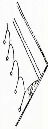
fig. 3.4.1 Fabric strip at the edge of the membrane
