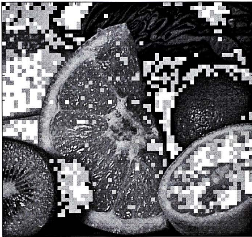
Figure 3.6: The locations of those blocks using joint optimization (white blocks) and those estimated by predictive coding (light-gray blocks) of image Fruits in the proposed estimation scheme using the conventional PIFS.
