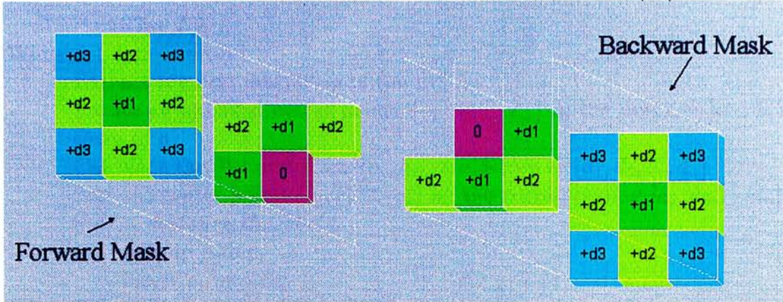
Figure 6.2: Masks for the three dimensional distance transform algorithm
