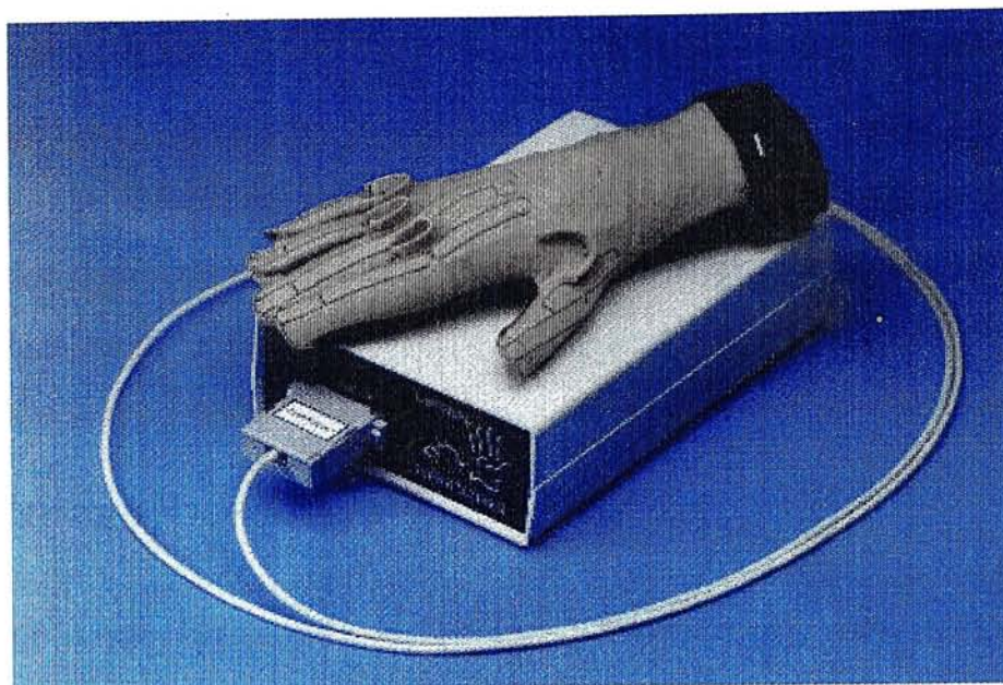
Figure 2.2. An 18-sensor CyberGlove and the CyberGlove Interface Unit (CGIU), which is responsible for the amplification and digitization of the sensor signals of the CyberGlove. (Picture adapted from http://www.virtex.com/ , the official homepage of Virtual Technologies.)
