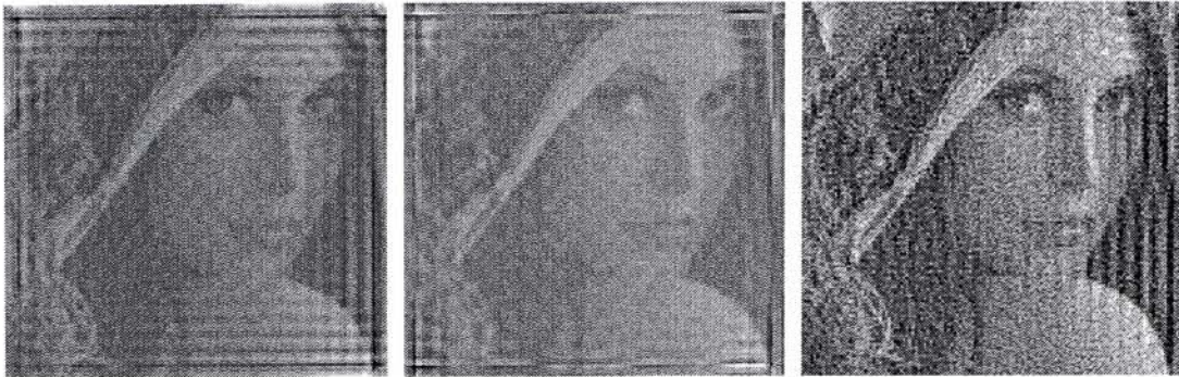
Figure 9: Restoring out-of-focus blur with zero boundary (left), periodic boundary (middle) and Neumann boundary (right) conditions, and \mu chosen by L-curve.
