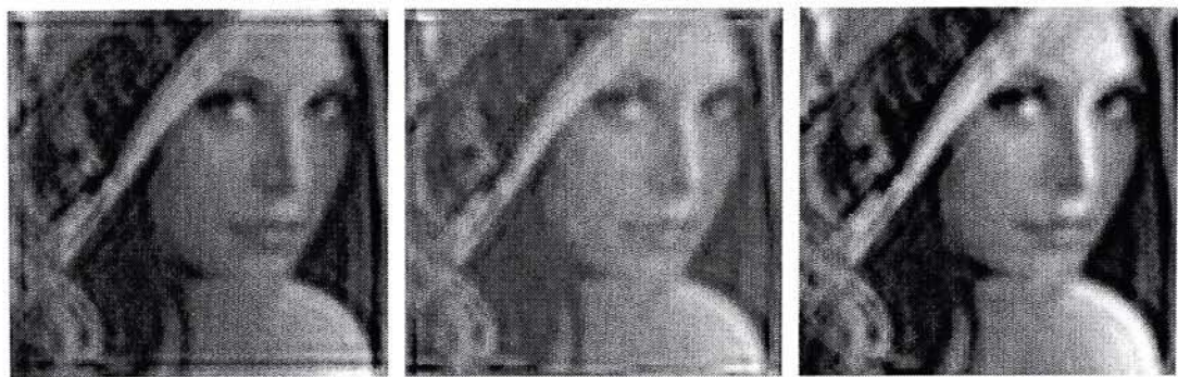
Figure 10: Restoring out-of-focus blur with zero boundary (left), periodic boundary (middle) and Neumann boundary (right) conditions, and \mu chosen visually.
