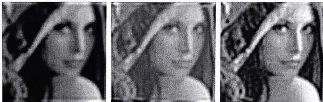
Figure 8: Restoring Gaussian blur with zero boundary (left), periodic boundary (middle) and Neumann boundary (right) conditions, and \mu chosen visually.
