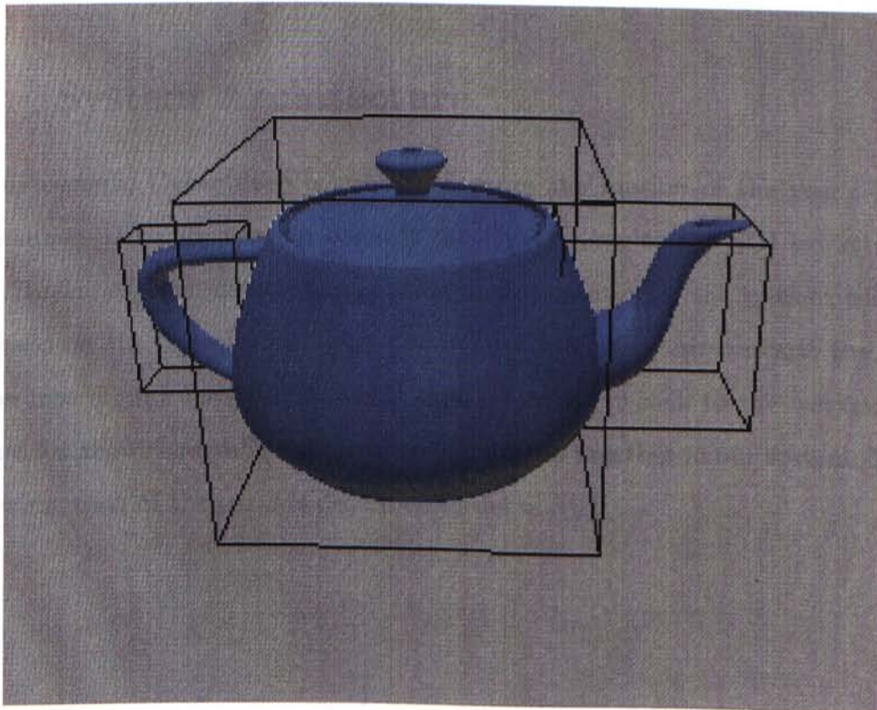
Figure 8.9: Teapot bounded by hierarchical primitives
