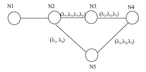
Figure 7c. Wavelength assignment after a lightpath is setup by using  $\lambda_4$  on the path  $r_{325}$  when SPA is used.
