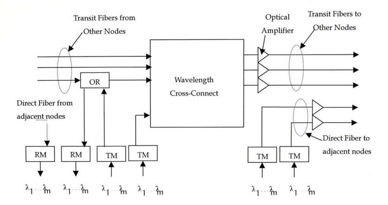
Figure 4. The proposed node architecture, where OR is the optical relay.
