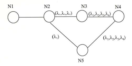
Figure 7b Wavelength-assignment after a lightpath is setup by using  $\lambda_4$  on the path  $r_{345}$  when MVA is used.
