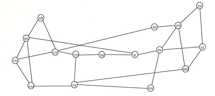
Fig.14. Physical topology of the NSFNET backbone network.
