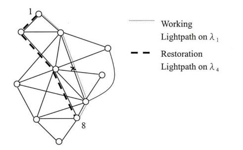
Figure 13. Source based restoration for the working lightpath between node 1 and node 8 by setting up a new lightpath not passing through the cut edge.
