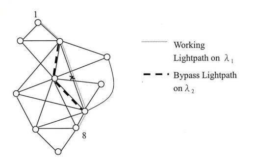
Figure 12. Link based restoration for the working lightpath between node 1 and node 8 by bypassing the cut edge.
