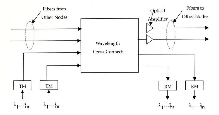
Figure 3. The conventional node architecture, where TM is transmitter module and RM is receiver module.
