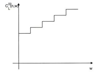
Figure 8. Typical fiber installation cost as a function of fiber number w.
