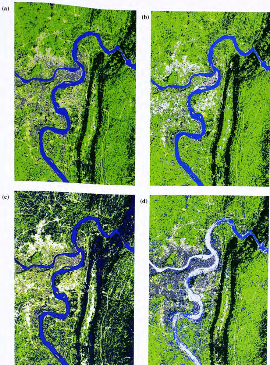
Figure 5.4 Classified images of Chongqing using different approaches: Object-oriented classification (a), maximum-likelihood classification (b), supervised fuzzy classification (c) and linear spectral unmixing (d)
