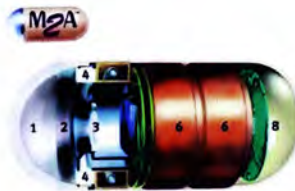
Figure 1-4 Composition of the M2A capsule: 1-Optical dome; 2-Lens holder; 3-Lens; 4-Illuminating LEDs; 5-CMOS imager; 6-Battery;7-Transmitter; 8-Antenna [6]
