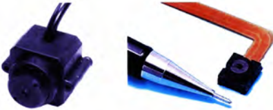
Figure 6-3 Left: A standard CMOS analog camera; Right: Fujitsu MB86S02A CMOS digital camera
