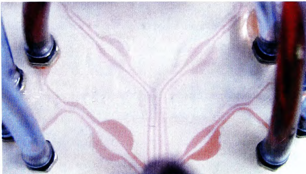
Figure 41. Fluid Pattern of the microchambers pumped with DI water (inlets B and D) and red dye (inlets A and C)
