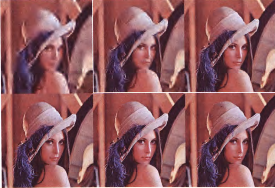
Figure 2.10: A color image sequence(size: 256 \times 256 , 24 bits per pixel)produced by the SPIHT method (bytes received: 505, 1126, 3789, 14746, 41472, 65536).
