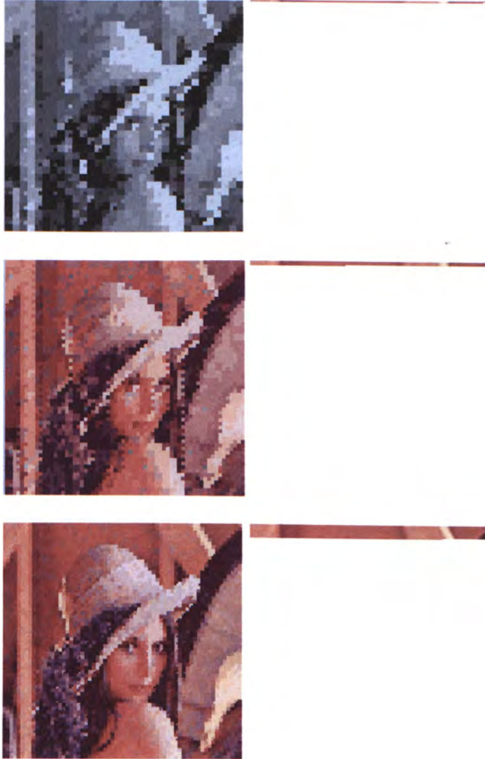
Figure 1.1: Image display in scanline order and progressive scan (bytes received order: 505, 1126, 3789, 14746, 41472, 65536)
