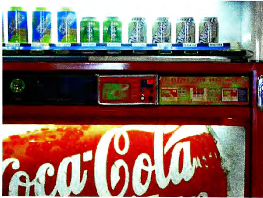
Figure 1.1: Octopus Card Payment System used in drink machine
