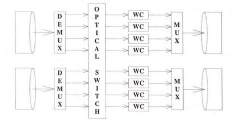
Figure 2.4: Schematic of the multi-fiber optical switch.
