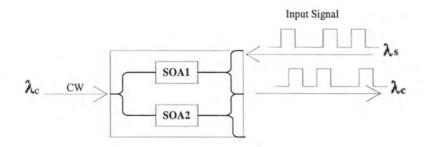
Figure 2.7: Schematic diagram of a wavelength converter based on XPM.
