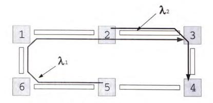
Figure 1.1: Wavelength routing in a ring network.
