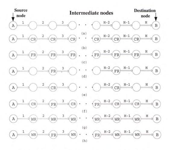
Figure 3.4: The paths with different reconfiguration capabilities.
