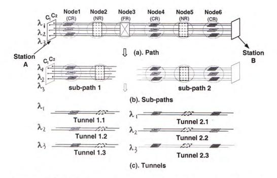
Figure 3.5: The decomposition procedure for the path with CRs, NRs, FR.
