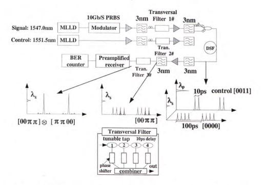
Figure 2.12: Experimental setup of optical code converter of scheme2.
