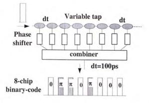
Figure 2.8: Experimental setup of optical code converter of scheme3.
