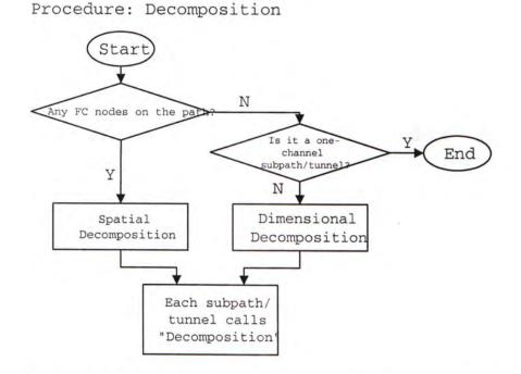
Figure 4.2: The flowchart of the iterative decomposition procedure for the inclusive converted network.
