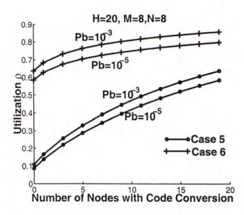
Figure 3.9: Link utilization versus number of nodes with code conversion. Pb: allowed blocking probability.
