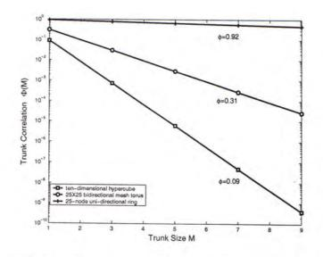
Figure 5.3: Traffic correlation versus the trunk size in a trunk switched network.
