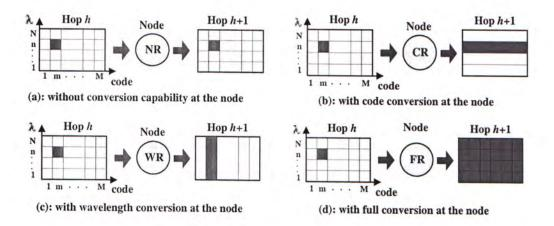
Figure 3.1: Possible channels for conversion to establish connections on the adjacent hops in a code/wavelength routing network.
