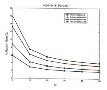
Figure 5.4: Utilization gain by multiplexing versus the original channel number for the networks with different link correlation.
