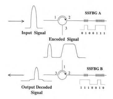
Figure 2.9: Outline of the physical approach of pulse encoding and decoding using superstructured fiber Bragg gratings (SSFBGs).
