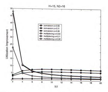
Figure 5.8: Utilization improvement (by multiplexing or by conversion) versus N1.
