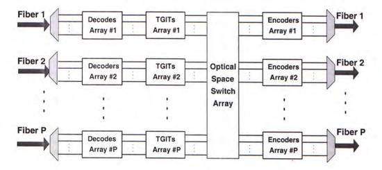
Figure 2.10: A proposed schematic of the OXC in a OCDM/WDM network.
