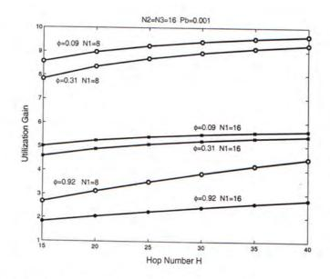
Figure 5.5: Utilization gain by multiplexing versus hop numbers for the networks with different original channel number  $N_1$ .
