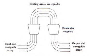
Figure 2.1: Top view of a typical arrayed waveguide grating used as a highly versatile passive WDM device.
