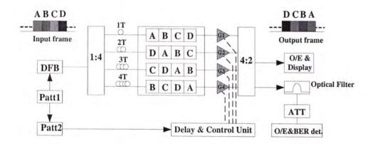
Figure 2.13: Schematic diagram of optical TSI experimental system.
