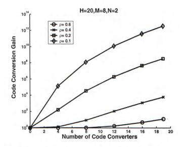
Figure 3.7: The code conversion gain versus the number of code converters along the path.
