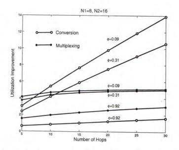
Figure 5.7: Utilization improvement (by multiplexing or by conversion) versus number of hops H.
