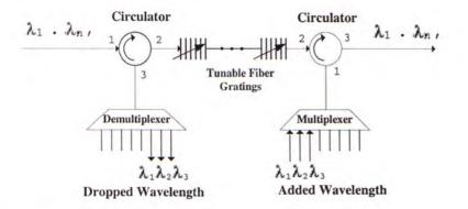
Figure 2.3: Multiple tunable filter grating used in conjunction with two optical circulators to add and drop any number of Ndifferent wavelengths.
