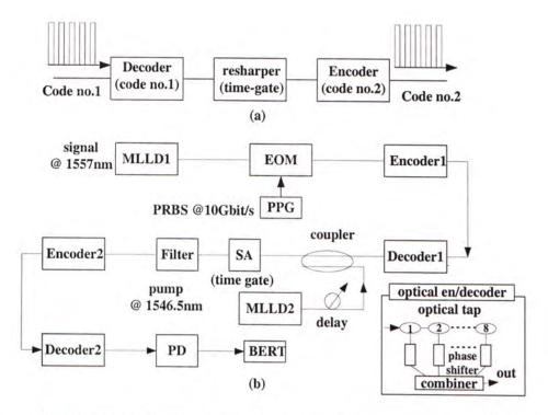
Figure 2.11: Experimental setup of optical code converter of scheme1.
