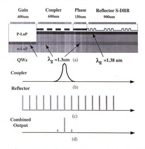
Figure 2.2: Schematic diagram of a three-section tunable distributed feedback (DFB) laser.
