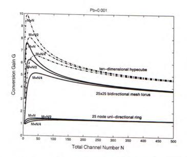
Figure 5.6: Conversion gain versus total number of channels.
