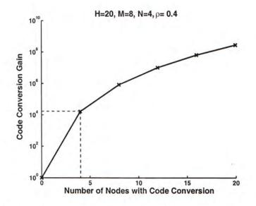
Figure 3.8: The code conversion gain when code conversion is sparsely added to the path already has WCs.
