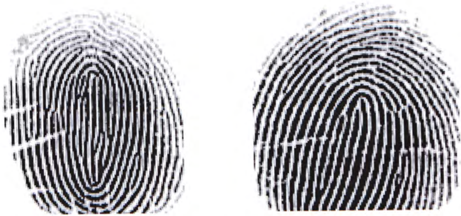
Figure 4.1 Fingerprint images acquired using the StarTek FM100 sensor (White areas: valleys; Black areas: ridges. The ridges are thicker than valleys.).
