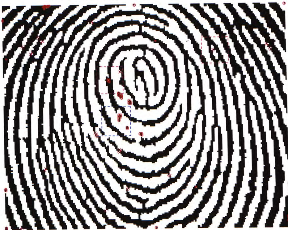
Figure 4.8 Preprocessing results at different processing steps. (Red cross: eliminated diagonal pixels; Red dots: filled pixels; Red circles: removed pixels).
