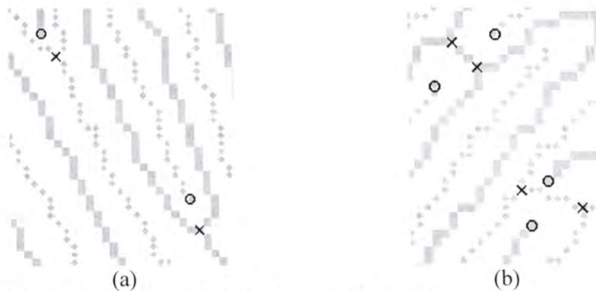
Figure 5.2 Illustration of ridge and valley duality. The solid gray squares represent the valley skeleton, and the solid gray diamonds represent the ridge skeleton. (a) The termination/bifurcation duality; (b) H -point examples: a valley bridge corresponds
