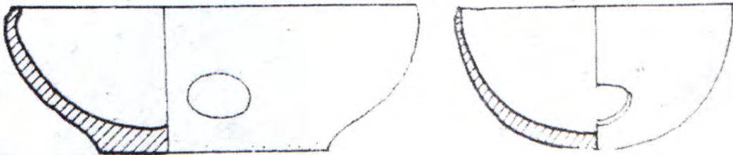
Fig. 3 -8a, 8b Bowl-shape temperature indicator used by the Changsha wares potters during firing. Hunan Provincial Museum Collection, 1996, fig. 309, 311.
