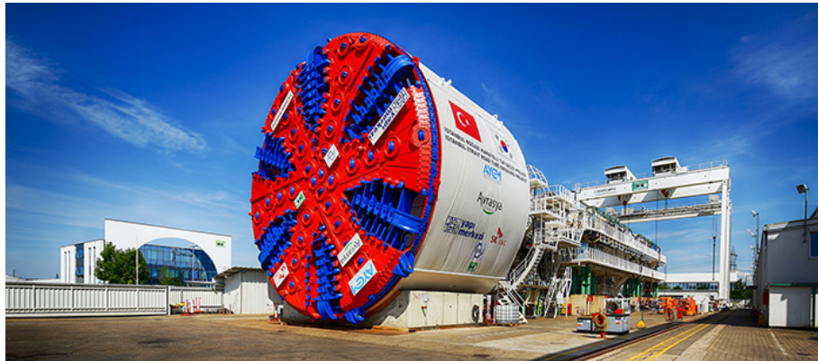
FIGURE 1.45 Tunneling machine Yıldırım Bayezid (DN:13,7 m) for The Eurasia Tunnel. (Source: www.avrasyatuneli.com/kurumsal/galeri/fotograf/tbm-tunel-acma )
