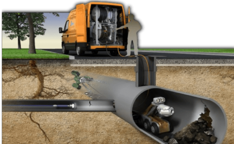
FIGURE 2.17 Closed-circuit television (CCTV) inspection. (Source: ISTT.)
