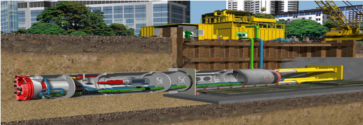
FIGURE 1.37 Machinery of microtunneling. (Source: ISTT)
