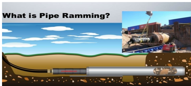
FIGURE 1.48 Pipe ramming and spoils. (Source: ISTT.)
