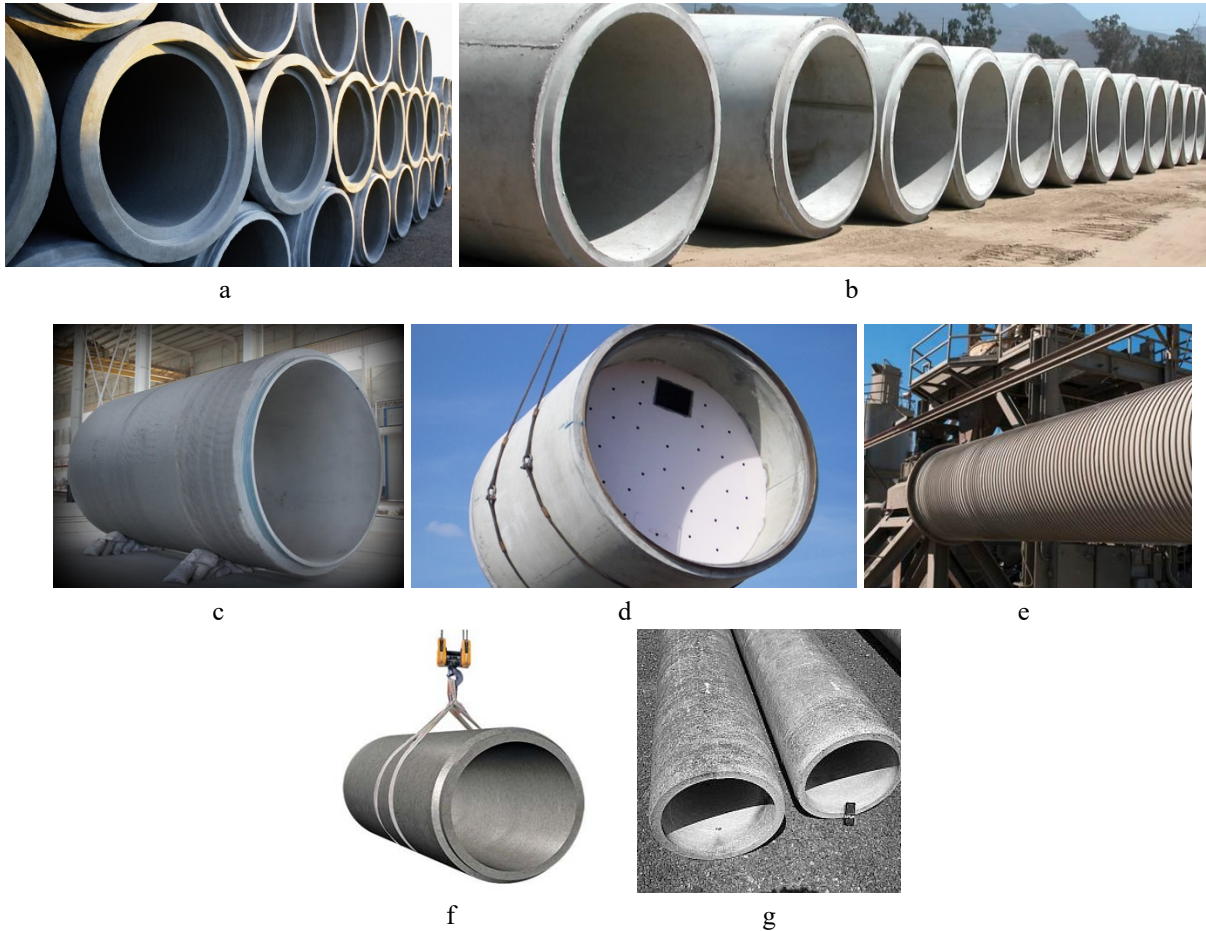
FIGURE 3.13 Concrete pipes a) Nonreinforced concrete pipes, b) Reinforced concrete pipes, c) Prestressed concrete cylinder pipe, d) Reinforced concrete cylinder pipe, e) Bar-wrapped steel-cylinder concrete pipe, f) Polymer concrete pipe, g) Asbestos-Cement Pipes. (Source: ISTT .)
