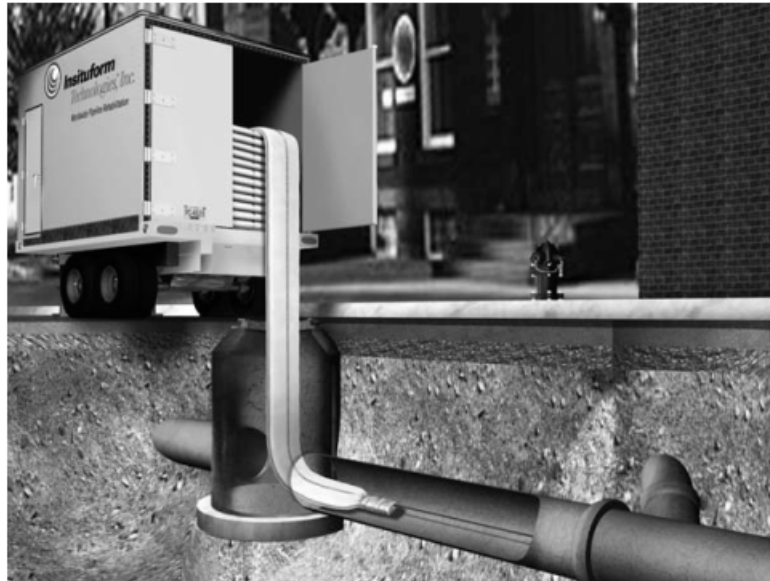
FIGURE 2.26 CIPP installation process. (Source: Insituform Technologies.)
