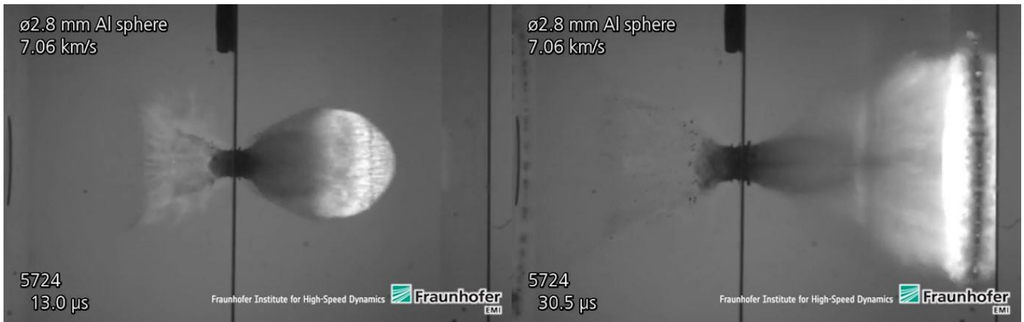
Figure 6: Whipple Shield 13 \mu s After Impact
