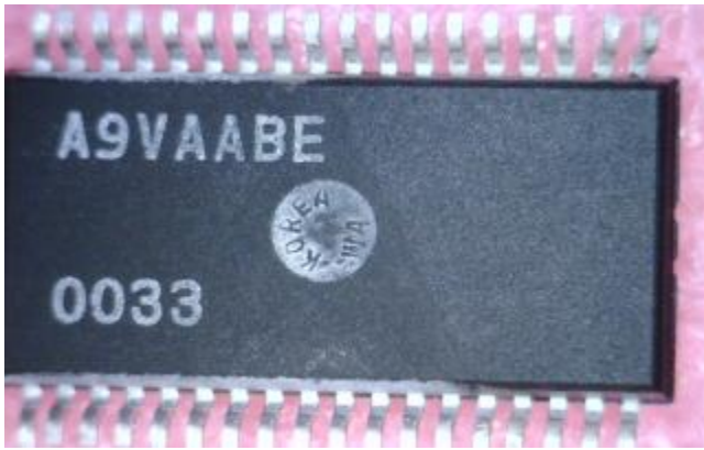
Figure 4: Counterfeit Part after Dynasolve
