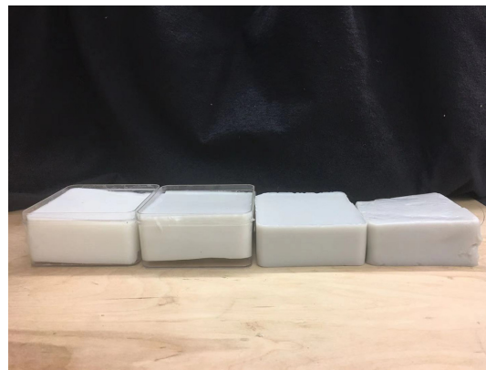
Fig. 4 Four high contrast solid phantoms for mimicking the chest wall with the size of 10 cm by 10 cm by 4 cm. Their absorption coefficients range from 0.095 to 0.18, and their reduced scattering coefficients range from 5.6 to 7.1 cm -1 .
