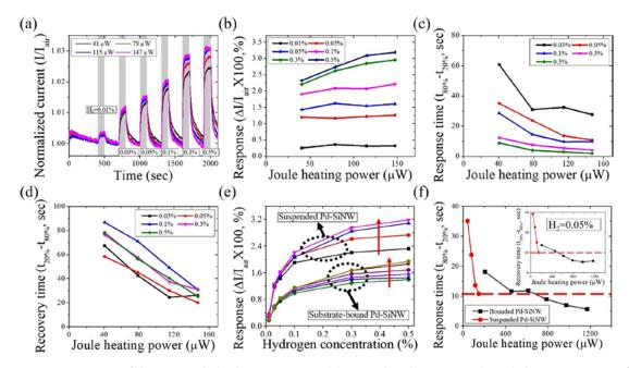
Figure 13.  $H_2$  gas sensing of the suspended Pd-SiNW sensor: (a) normalized current with Joule heating powers of 41, 79, 115, and 147  $\mu$ W. The (b) response, (c) response time and (d) recovery time for variant  $H_2$  concentrations at four Joule heating powers. Comparison between the substrate-bound and suspended Pd-SiNW sensors: (e) responses at various Joule heating powers (red arrows: direction of Joule heating power increment (from 41 to 147  $\mu$ W for the suspended Pd-SiNW
