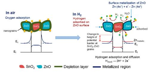
Figure 33. The schematic diagram for explanation of sensing mechanism of  $ZnO-SnO_2$  heterojunction [140]. Copyright (2015), with permission from American Chemical Society.
