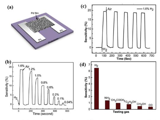
**Figure 6.** The hydrogen response of nanoporous Pd film sensors at room temperature. (a) The transient response to various concentrations of  $H_2$  in the air; (b) the H2 concentration-dependent response time and sensitivity; (c) repeatability; (d) selectivity [58]. Copyright (2016), with permission from Elsevier.
