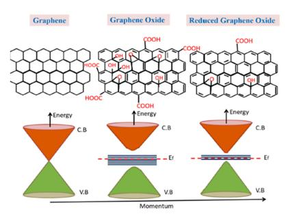
**Figure 35.** Schematic representation of lattice structure and corresponding energy diagrams of graphene, graphene oxide (GO) and reduced graphene oxide (rGO) [149]. Copyright (2018), with permission from Nature Publisher Group.
