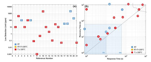
**Figure 34.** Regarding Table 2, schematic illustrations of the comparison of the reported: (a) low detection limits. The x-axis "Reference Number" represents the 1st column"Ref. Nr." in Table 2. (b) Response time/recovery time under experimental conditions in the literature.
