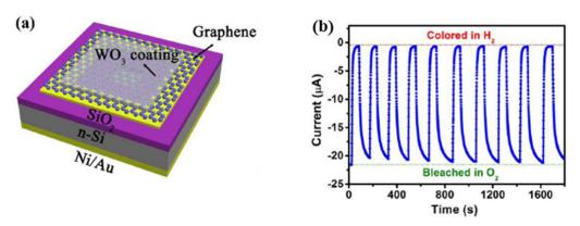
**Figure 46.** (a) Schematic of the optoelectronic Pd-WO<sub>3</sub>/Graphene sensor. (b) Cyclic performance of the device [209]. Copyright (2018), with permission from Elsevier.
