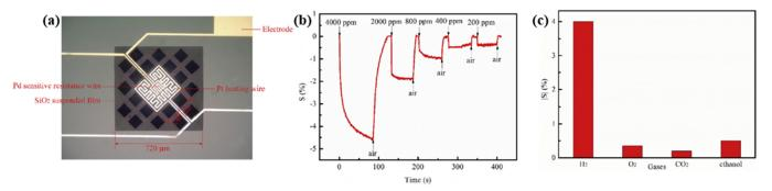
**Figure 7.** (a) Microscope image of a hydrogen sensor sample. (b) Responses of different H<sub>2</sub> concentrations at 400 °C, and (c) responses of the sensor to various gases (4000 ppm) at 400 °C [59]. Copyright (2019), with permission from Elsevier.
