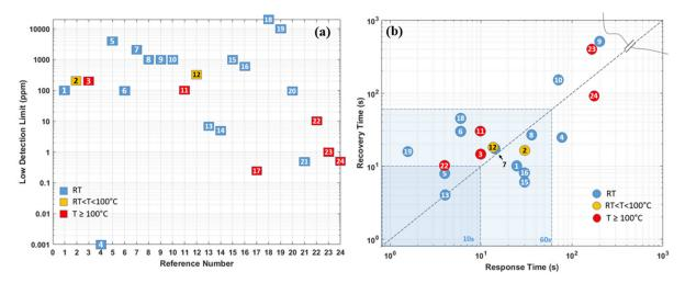
**Figure 18.** Regarding Table 1, schematic illustrations of the comparison of the reported Pd-based hydrogen gas sensors in literature: (a) low detection limits. The x-axis "Reference Number" represents the 1st column"Ref. Nr." in Table 1. (b) Response time/recovery time under experimental conditions as reported in the literature.
