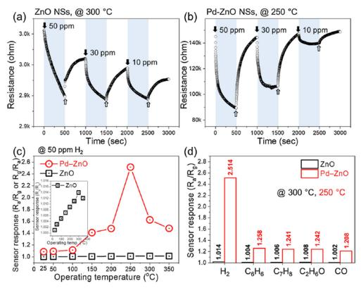
**Figure 29.** Dynamic resistance curves of (a) pristine and (b) Pd-decorated ZnO nanosheets to  $H_2$  gas. (c) The response of pristine and Pd-decorated ZnO nanosheets to 50 ppm of  $H_2$  gas at different sensing temperatures. The inset shows the response of a pristine sensor to  $H_2$  gas and (d) selectivity patterns of ZnO and Pd-decorated ZnO nanosheet at optimal temperatures [122]. Copyright (2021), with permission from Elsevier.
