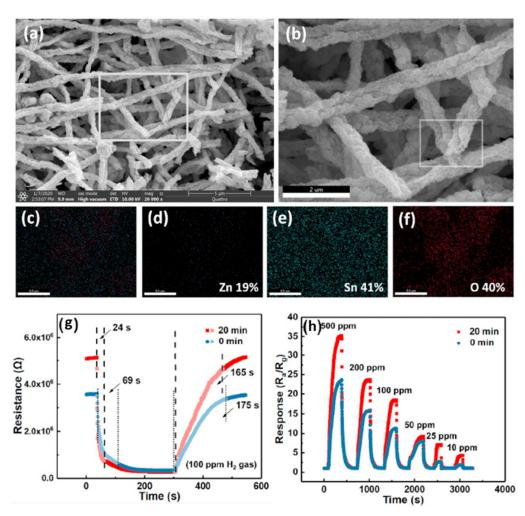
**Figure 32.** (**a**,**b**) SEM images of ZnO–SnO<sub>2</sub> nanofibers, (**c**-**f**) images of area scan by EDS including the element content of Zn, Sn, and O. (**g**) Response and recovery at optimum operating temperature 300 °C. (**h**) Response curve with 10 ppm to 500 ppm H<sub>2</sub> concentrations at an optimum operating temperature [123]. Copyright (2020), with permission from Elsevier.
