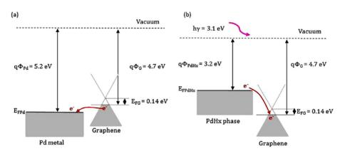
**Figure 36.** Energy band diagrams (**a**) for Pd decorated graphene and (**b**) for PdH<sub>x</sub> and graphene [162]. Copyright (2019), with permission from Nature Publisher Group.
