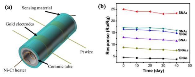
**Figure 26.** (a) Schematic diagram of SnO<sub>2</sub> gas sensing element. (b) Long-term stability of the prepared gas sensors to 100 ppm H<sub>2</sub> at their optimum temperatures [115]. Copyright (2017), with permission from Elsevier.
