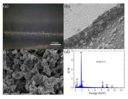
**Figure 31.** (a) Morphology of double spiral microstructure after depositing Pt-WO<sub>3</sub> film. (b) The cross-section diagram of Pt-WO<sub>3</sub> film. (c) The SEM picture of nanostructure of Pt-WO<sub>3</sub>. (d) The energy-dispersive X-ray spectrometer (EDS) pattern of Pt-WO<sub>3</sub> film [136]. Copyright (2017), with permission from OPTICA Publishing Group.
