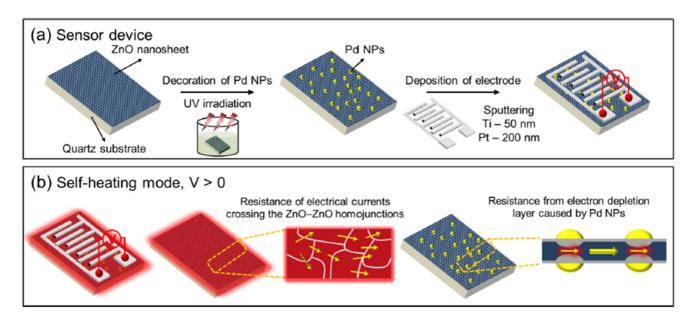
**Figure 28.** (a) Schematic of sensor fabrication and (b) operation in self-heating mode [122]. Copyright (2021), with permission from Elsevier.
