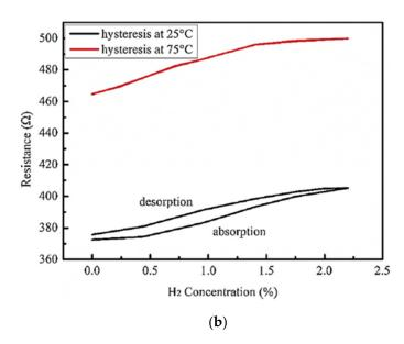
**Figure 4.** (a) The optical microscope image of the Pd/Ni sensor and (b) the hysteresis of hydrogen absorption and desorption at 25 °C and 75 °C [37]. Copyright (2019), with permission from Elsevier.
