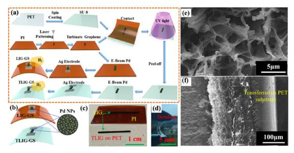
Figure 41. (a) The fabrication process of the laser-induced graphene gas sensor (LIG-GS) and transferred LIG-gas sensor (TLIG-GS). (b) Schematic of Pd NPs on LIG-GS and TLIG-GS. (c) Transferred line pattern of 3D porous LIG. (d) Image of bendable TLIG-GS. (e) Morphology of TLIG and (f) cross-sectional image of TLIG [180]. Copyright (2019), with permission from American Chemical Society.
