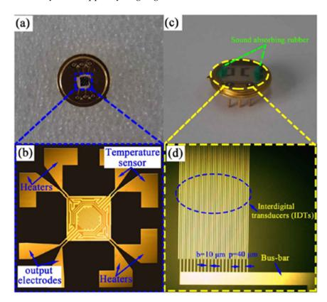
**Figure 25.** Two kinds of hydrogen gas sensors based on SnO<sub>2</sub> films: (a) the chemi-resistive hydrogen gas sensor, (b) the micrograph of the chemi-resistive hydrogen sensor, (c) the delay-line surface acoustic waves (SAW) hydrogen gas sensor, and (d) the micrograph of interdigital transducers (IDTs) of the SAW hydrogen sensor [112]. Copyright (2017), with permission from Elsevier.
