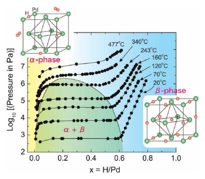
**Figure 2.** H<sub>2</sub> pressure–composition–temperature (P–C–T) phase diagram of the Pd-H system [22,23]. Copyright (2019), with permission from Chemistry Europe.
