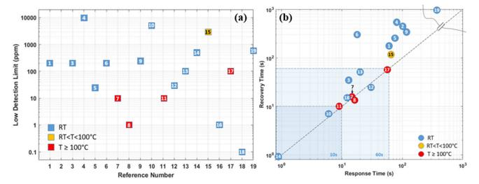
**Figure 42.** Regarding Table 3, schematic illustrations of the comparison of the reported: (a) low detection limits. The x-axis "Reference Number" represents the 1st column"Ref. Nr." in Table 3. (b) Response time/recovery time under experimental conditions in literature.
