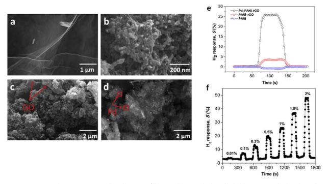
**Figure 38.** Scanning electron microscope (SEM) images of (a) rGO, (b) PANI (polyaniline), (c) PANI-rGO (reduced graphene oxide) and (d) Pd-PANI-rGO. (e) Gas sensing response of the PANI, PANI-rGO and Pd-PANI-rGO thin films exposed to 1% hydrogen concentration at room temperature. (f) Gas sensing response of the Pd-PANI-rGO based sensor to different concentrations of hydrogen at room temperature [176]. Copyright (2016), with permission from Elsevier.
