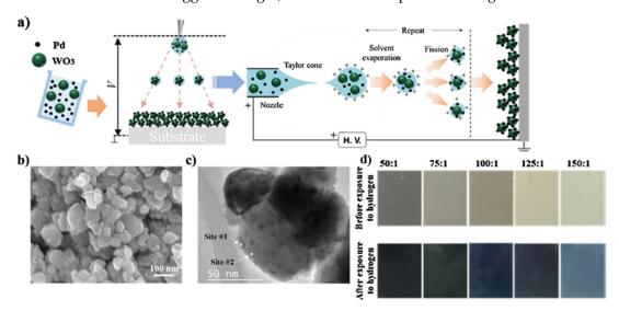
**Figure 30.** (a) Schematic of electrostatic spray deposition (ESD) process for fabricating WO<sub>3</sub>-Pd sensor, (b) SEM image of deposited WO<sub>3</sub>-Pd layer with a WO<sub>3</sub>:Pd ratio of 75:1, (c) TEM image of WO<sub>3</sub>-Pd, and (d) optical images of sensors with WO<sub>3</sub>:Pd ratios of 50:1, 75:1, 100:1, 125:1 and 150:1 before and after exposure to 1% hydrogen gas [131]. Copyright (2021), with permission from Elsevier.
