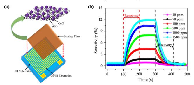
**Figure 45.** (a) Structure illustration of CuO-rGO-CuO hydrogen sensor, and (b) response–recovery curves for various concentrations of hydrogen [202]. Copyright (2017), with permission from Springer.
