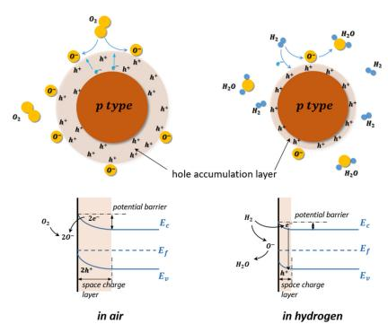
**Figure 20.** Schematic illustration of the gas sensing mechanism of p-type MOS and its energy band change in the air and hydrogen.
