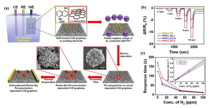
**Figure 40.** (a) Illustrative diagram for the fabrication steps of flower-like Pd nanoclusters (FPNCs) on chemical vapour deposition (CVD) graphene electrode. (b) Normalized resistance changes upon sequential exposure to H<sub>2</sub> gas of various concentrations (0.1 to 100 ppm) at room temperature, and (c) response time and rate (inset) vary with H<sub>2</sub> concentration [179]. Copyright (2015), with permission from Nature Publisher Group.
