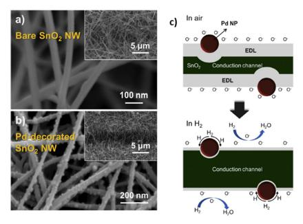
**Figure 17.** Field-emission scanning electron microscope (FE-SEM) micrographs of (a) bare SnO<sub>2</sub> NWs and (b) Pd-decorated SnO<sub>2</sub> NWs. Upper-right inserts are the top-view of the FE-SEM images. (c) The sensing mechanism of Pd-decorated SnO<sub>2</sub> NWs [87]. Copyright (2017), with permission from Elsevier.
