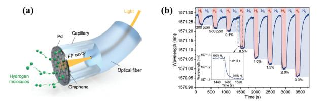
**Figure 39.** (a) Schematic of a fibre-optic H<sub>2</sub>-sensor with Pd-decorated MLG film, and (b) temporal response of the Pd/MLG sensor with a 5.6 nm Pd film for various H<sub>2</sub> concentrations [163]. Copyright (2019), with permission from Royal Society of Chemistry.
