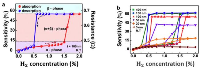
**Figure 3.** Hysteresis curve of sensitivity during the process of absorption and desorption of hydrogen from 0 to 2% concentration (**a**) for the Pd thin film with the thickness of 100 nm and (**b**) for the Pd thin film with thicknesses ranging from 5 to 400 nm [26]. RT means room temperature. Copyright (2010), with permission from Elsevier.
