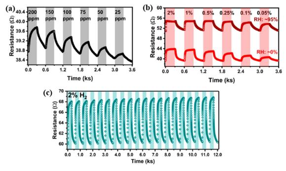
**Figure 37.** (a) Sensitivity of Pd-CGB sensor at ppm levels of  $H_2$  concentration from 25 to 200 ppm. (b) Effect of humidity on the sensor performance at two relative humidity (RH) levels: RH~0% and RH~95%. (c) Repeatability test of Pd-CGB sensor at 2%  $H_2$  for 20 cycles [170]. Copyright (2020), with permission from American Chemical Society.
