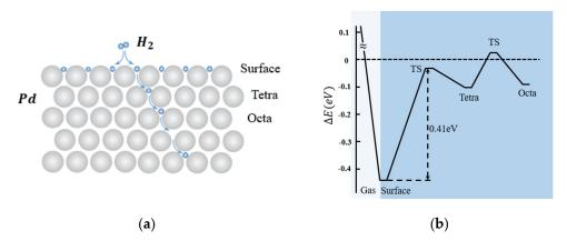
**Figure 1.** (a) Illustration of hydrogen adsorption in Pd (100) [16]; (b) diagram of the potential energy profile of hydrogen-absorption [17]. Copyright (2017), with permission from American Chemical Society.
