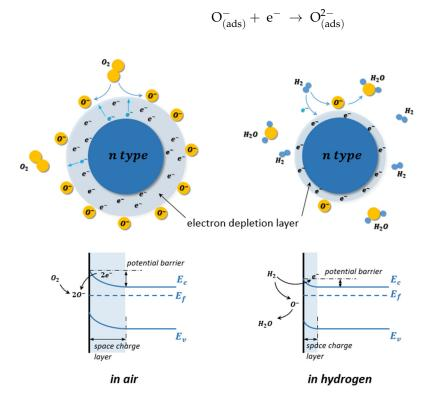
**Figure 19.** Schematic illustration of the gas sensing mechanism of n-type metal oxide semiconductor (MOS) and its energy band change in the air and hydrogen.
