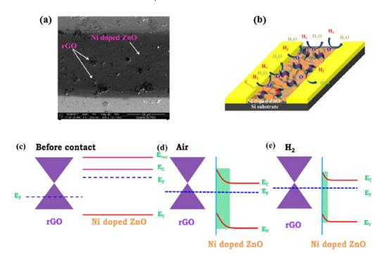
**Figure 43.** (a) SEM image of Ni-doped ZnO nanostructure and 0.75 wt% rGO loaded ZnO. (b) Schematic diagram of the gas sensing mechanism in the presence of hydrogen, (c–e) The band diagram illustration of rGO/ZnO heterojunction before contact and after contact in air and hydrogen) [198]. Copyright (2018), with permission from American Chemical Society.
