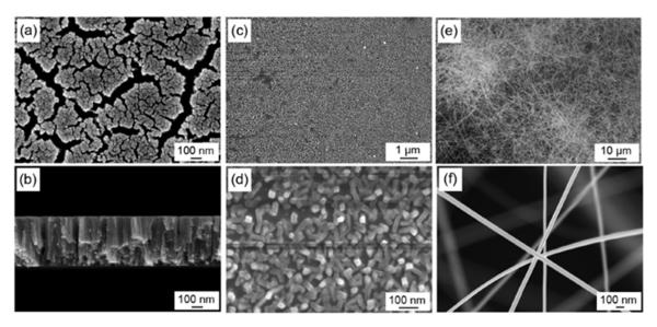
**Figure 21.** (a) Surface and (b) cross-sectional field of the emission scanning electron microscopy (FE-SEM) images of SnO<sub>2</sub> nanofilms. (c) Low- and (d) high-magnification FE-SEM images of SnO<sub>2</sub> nanorods. (e) Low- and (f) high-magnification FE-SEM images of SnO<sub>2</sub> nanowires [105]. Copyright (2015), with permission from Elsevier.
