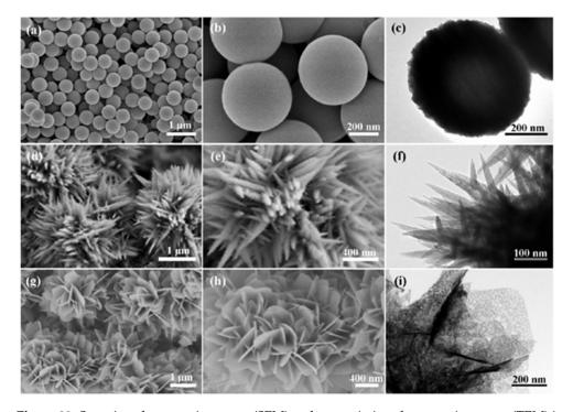
Figure 23. Scanning electron microscope (SEM) and transmission electron microscope (TEM) images of the  $SnO_2$  samples with different morphologies: (a–c) solid spheres (S0), (d–f) nano-needle assembled nano-urchins (S1), (g–i) nanosheet-assembled nanoflowers (S2) [106]. Copyright (2019), with permission from Elsevier.
