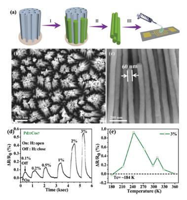
**Figure 10.** (a) Schematic for the synthesis and integration of PdCo nanowires (NWs) including (I) electrodeposition, (II) removal of anode aluminium oxide (AAO) and (III) integration. (b) The top-view and (c) side-view scanning electron microscope (SEM) images of PdCo NWs arrays. (d) The hydrogen sensing response of Pd33Co67 to 0.1–3%  $H_2$  at 273 K and (e) its temperature-dependent hydrogen response [64]. Copyright (2019), with permission from Royal Society of Chemistry.
