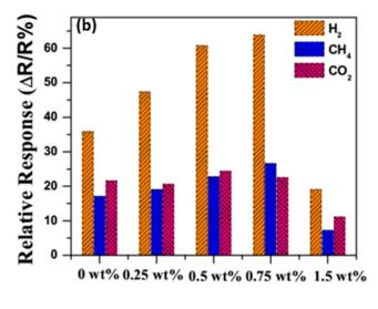
**Figure 44.** (a) Relative response of a 0.75 wt% rGO loaded sensor at an operating temperature of 150 °C with increasing gas concentration from 1 ppm to 100 ppm. (b) Selectivity histograms for pristine and rGO-loaded sensors with Ni-doped ZnO nanostructures [198]. Copyright (2018), with permission from American Chemical Society.
