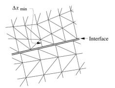
Figure 2. Dimension of zone used in stiffness calculation.
