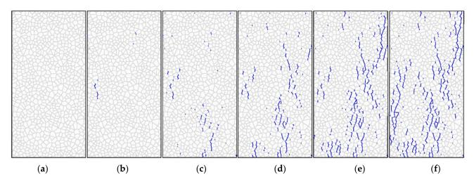
**Figure 10.** Development of tensile cracks in rock specimen in UDEC: (a) step 30,000; (b) step 60,000; (c) step 90,000; (d) step 120,000; (e) step 150,000; (f) step 180,000.
