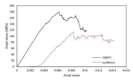
**Figure 7.** Stress-strain relationship for rock at  $1000\,^{\circ}$ C and post cool-down (reprinted from [26] with permission of Springer Nature).
