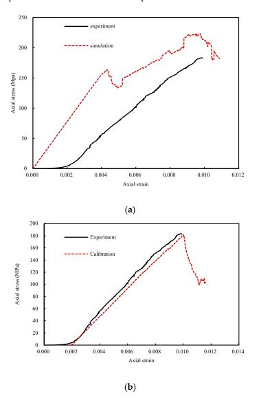
**Figure 3.** The strain-stress curves: (a) before calibration; (b) after calibration.
