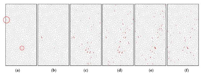
**Figure 9.** Development of shear cracks in rock specimen in UDEC: (a) step 30,000; (b) step 60,000; (c) step 90,000; (d) step 120,000; (e) step 150,000; (f) step 180,000.
