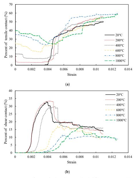
**Figure 13.** Percent of contact after being heat-treated with different temperature: (a) tensile contact; (b) shear contact.
