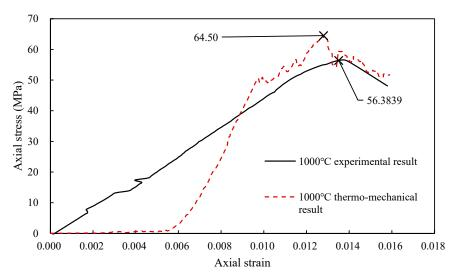
**Figure 5.** Comparison of experimental and predicted stress–strain relationships for rocks subjected to heat treatment at  $1000 \,^{\circ}$ C.
