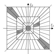
**Figure 4.** Illustration of the Fourier supports of the different components. (1) Coarse scaling part covering low frequencies. (2) Interior shearlets entirely contained in the interior of the cones. (3) Boundary shearlets "glued" together along the boundaries of the cones.
