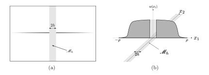
**Figure 6.** (a) Sketch of the corrupted modeling image. Note that the line singularity has no "thickness" but some (gray-scale) intensity. (b) "Graph" of the corrupted line distribution  $P_K \mathfrak{wL}$ , which is compactly supported on the  $x_1$ -axis.
