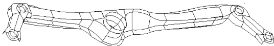
Figure 1: A coarse mesh modeling a chassis of a car. This mesh has been constructed by a German car company.
