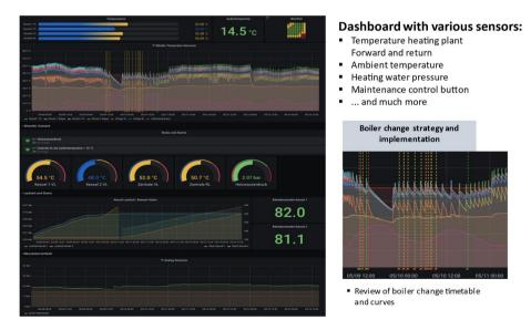
Fig. 5 Oktett64 real time measurement and metering including time-chart analysis
