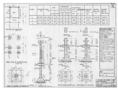
**Figure 9a:** Graphical Expression of the design and construction of R.C.C columns (Image Source: Authors).
