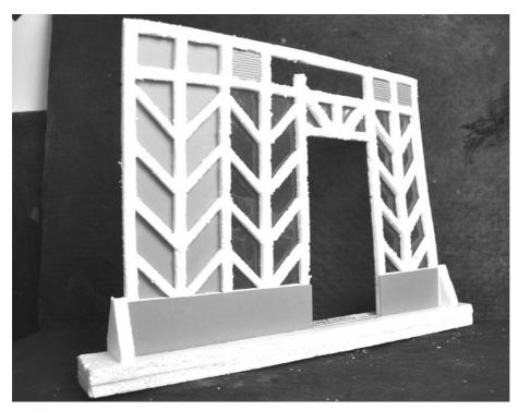
Figure 4: Experimental Model of a 'Timber Partition' designed and executed by students (Image Source: Authors).
