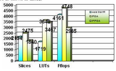
Figure 6: Area Comparison of Add Shift and PDA with PPDA
