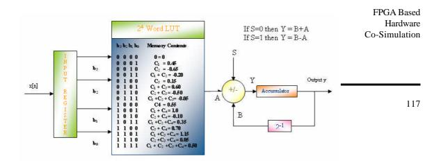
Figure 1: LUT based DA implementation of 4-tap filter LUT Unit: To implement 4-input and 3-input LUT unit, an LUT table is used, which represent all the possible sum combinations of filter coefficients Figure 1.
