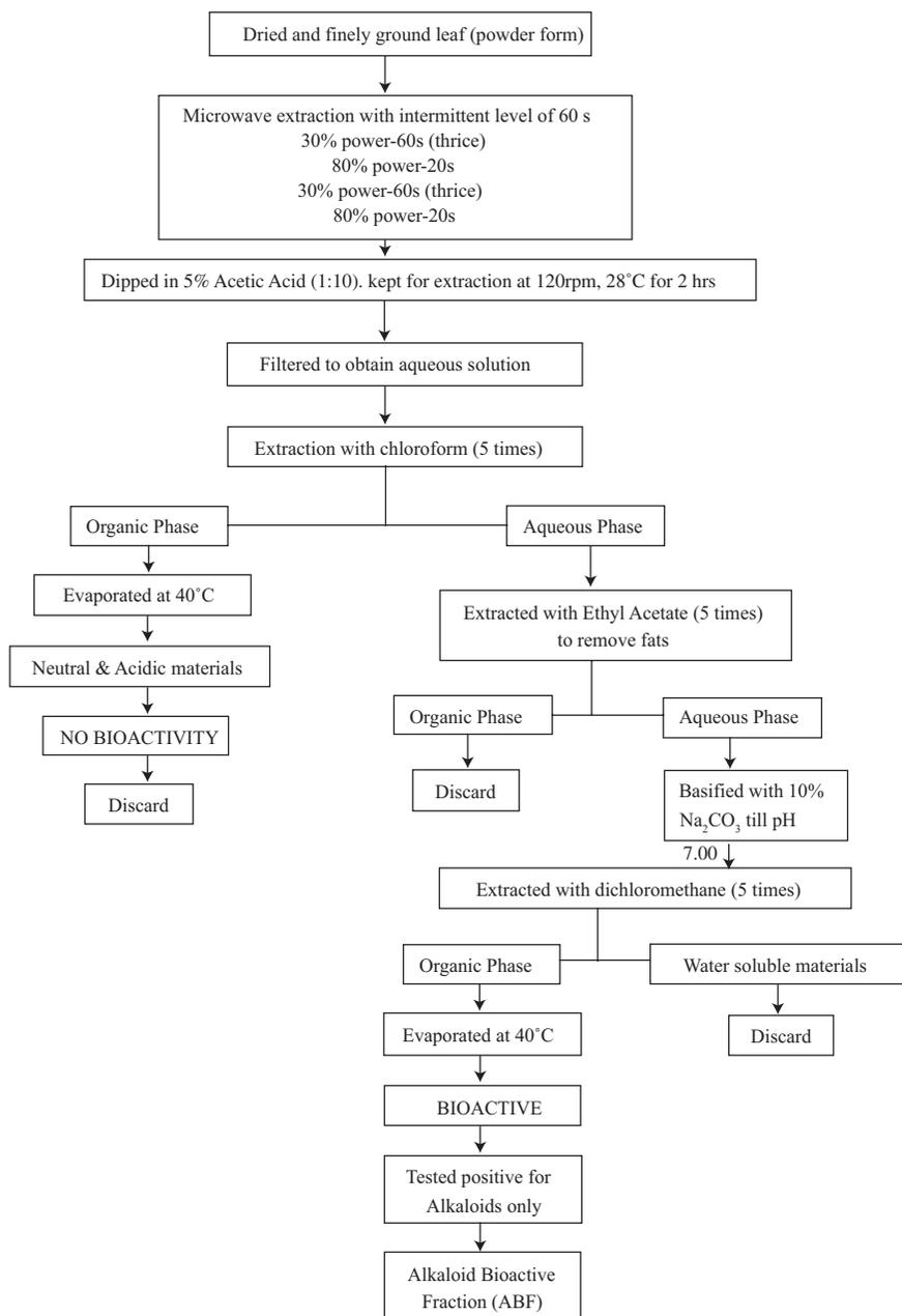
**Figure 1:** Schematic representation of extraction of Alkaloid Bioactive Fraction from *C. rigidus* leaves
