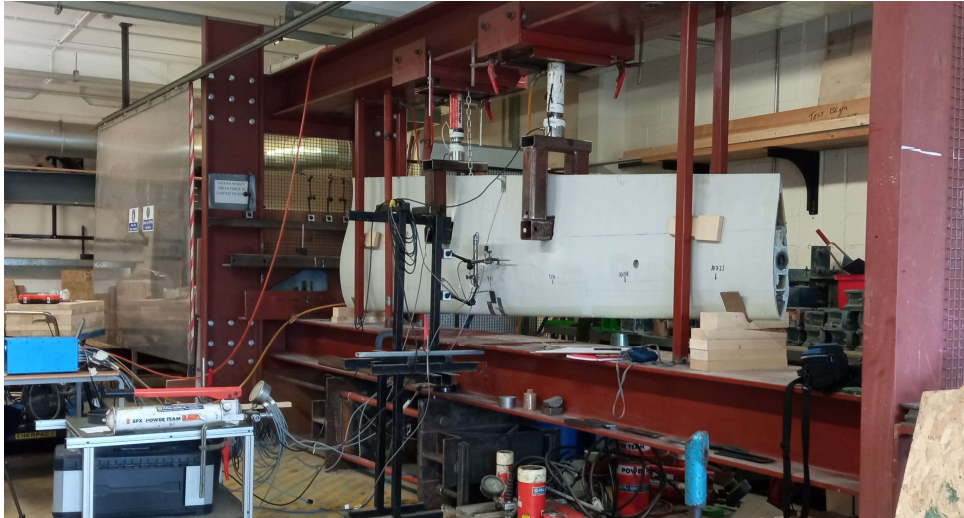
Figure 6. Load testing cell at the Structures Laboratory, MTU, showing N29 blade section under test.
