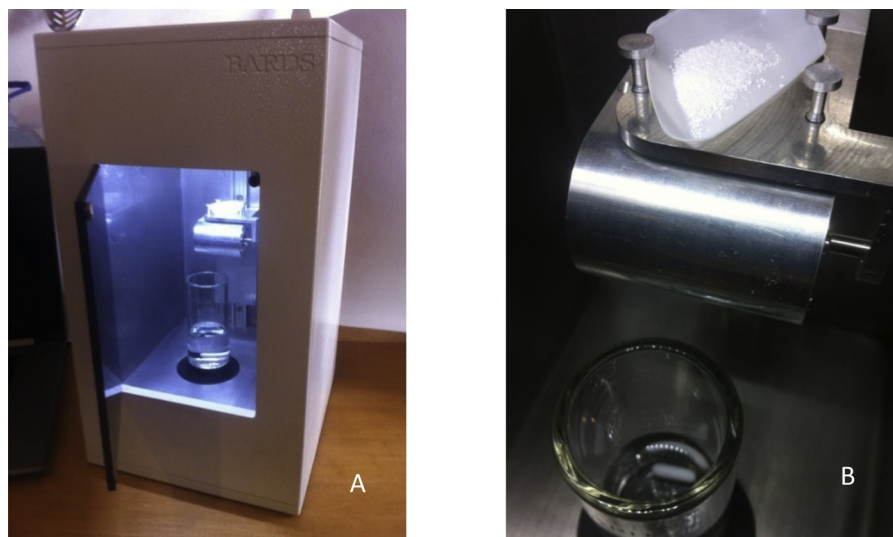
Fig. 1. (A) External view of the BARDS instrument and (B) Tipper motor with a sample of glucose in a weighing boat ready for addition to the stirring solution below, e.g. yeast suspension.
