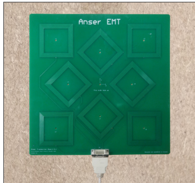
Figure 9. The field generator comprises a set of eight planar transmitter coils, as first presented in [12]. Each coil is driven with a sinusoidal current at a different frequency and the sensor coil uses frequency-division multiplexing (FDM) to distinguish the eight signals.
