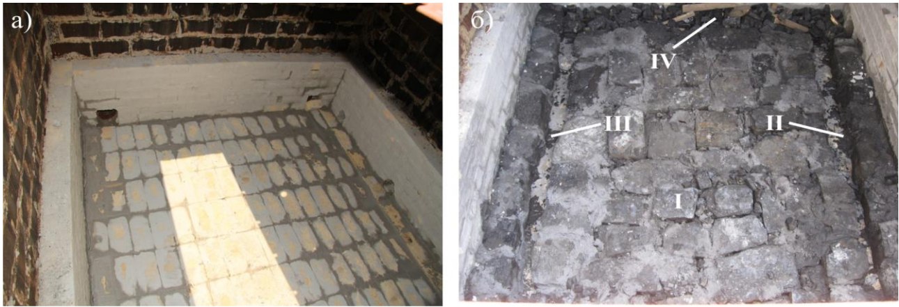
Fig. 2. Model of underground gasgenerator: a) heat-insulation of stand box; b) coal seam formation: I – a coal seam; II – a blowing borehole; III – a gas outlet borehole, IV– reactionary channel (imitation of hydrofracturing)
