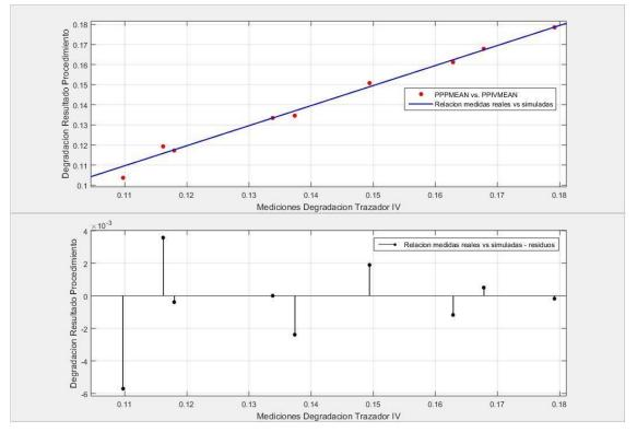
Figure 3. Relationship between the degradation resulting from the procedure and Tracer I-V 400.
