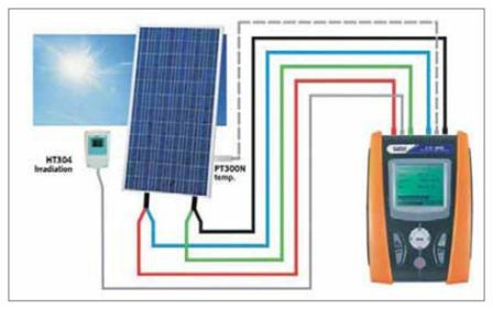
Figure 2. I-V 400 Curve Tracer
