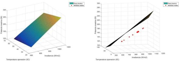
Figure 4. Theoretical behavior of the PV module 2 compared to the measurements carried out
