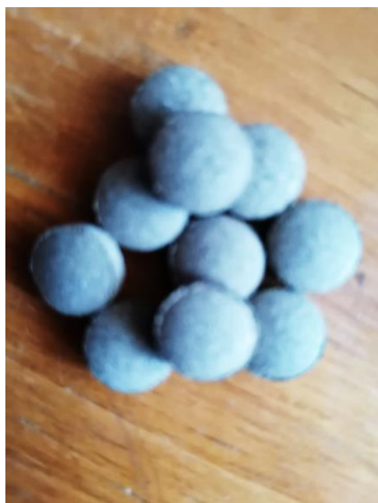
Figure 1. Raw pellets produced on the rotary disk pelletizer
