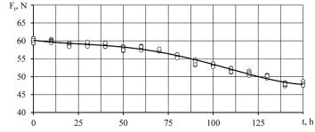
Fig. 5. Dynamics of the tensile strength of teat cup liner Ft(t) from the duration of operation
