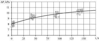
**Fig. 4.** Dynamics of the closing vacuum value  $\Delta P(t)$  from the duration of operation
