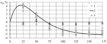
**Fig. 3.** Change in the mass of teat cup liner during periodic exposure to milk, acid detergent from Ekolat and water:  $1 - DD \ 00.041A$  teat cup liner made of rubber compound material produced by Bratslav OJSC;  $2 - \varepsilon_M(t) = -3.3 + 0.8(t - 4.8)\exp(-0.039 \cdot (t - 4.8))$ ; 3 - BouMatic teat cup liner (analogue of DD.00.041A) made of «BouMatic Robotics» food grade silicone
