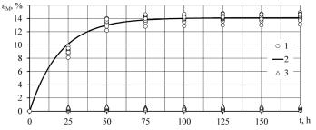
**Fig. 2.** Change in the mass of teat cup liner during continuous presence in milk: 1 – teat cup liner DD 00.041A from the material of rubber compound produced by JSC «Bratslav»; 2 – the equation  $\varepsilon_M(t) = 14.1(1-\exp(-0.051 \cdot t))$ ; 3 – BouMatic teat cup liner (analogue DD.00.041A) made of food-grade silicone material «BouMatic Robotics»
