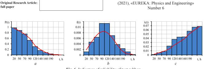
**Fig. 6.** Indicators of reliability of teat rubber: *a* – probability of failure-free operation P(t); *b* – failure rate  $\lambda(t)$ ; *c* – failure density f(t)
