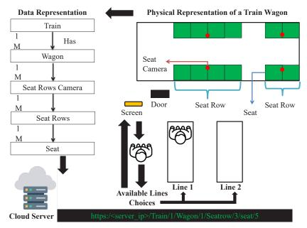
Fig. 2. Overview of the adaptive queue line system
