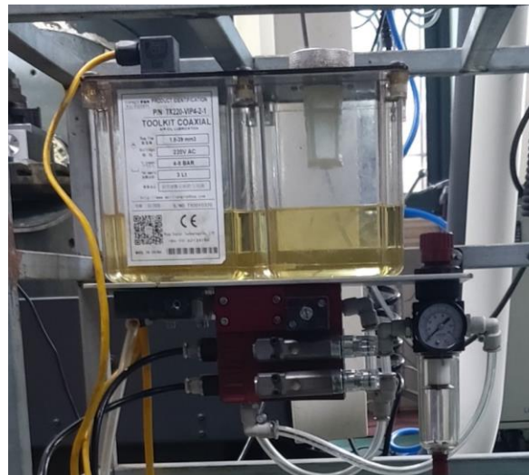
Fig. 3. Minimum Quantity Lubrication System
