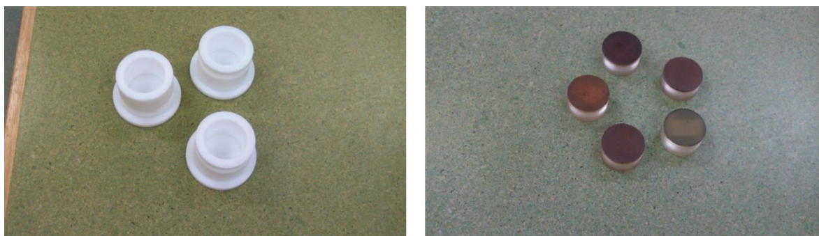
Figure 8. Photo of the sample holders (left) and polished resin blocks (right).
