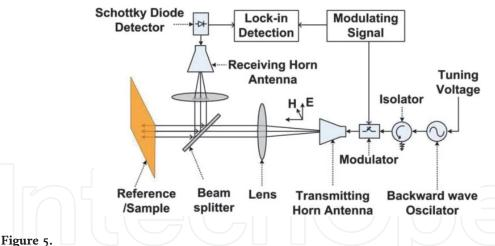
Measurement setup of the millimeter-wave absorber ([51], reproduced courtesy of The Electromagnetics Academy).
