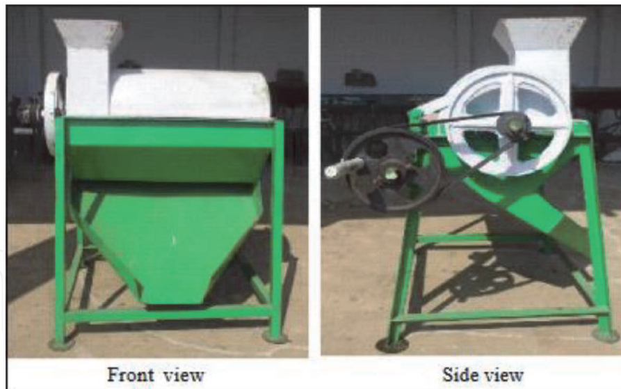
Figure 3. Manual maize sheller [18].
