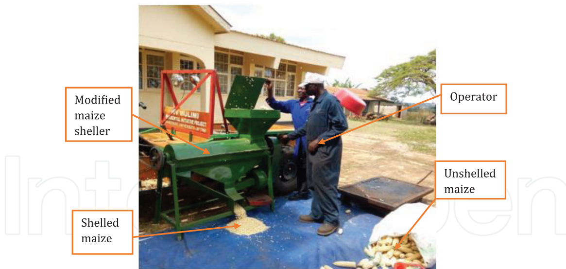
Figure 6. Operational view of the modified multi-purpose vehicle maize sheller [1].
