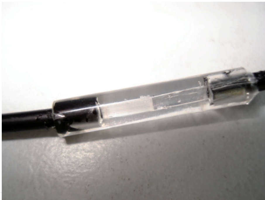
Figure 13. Optical splice with low attenuation.
