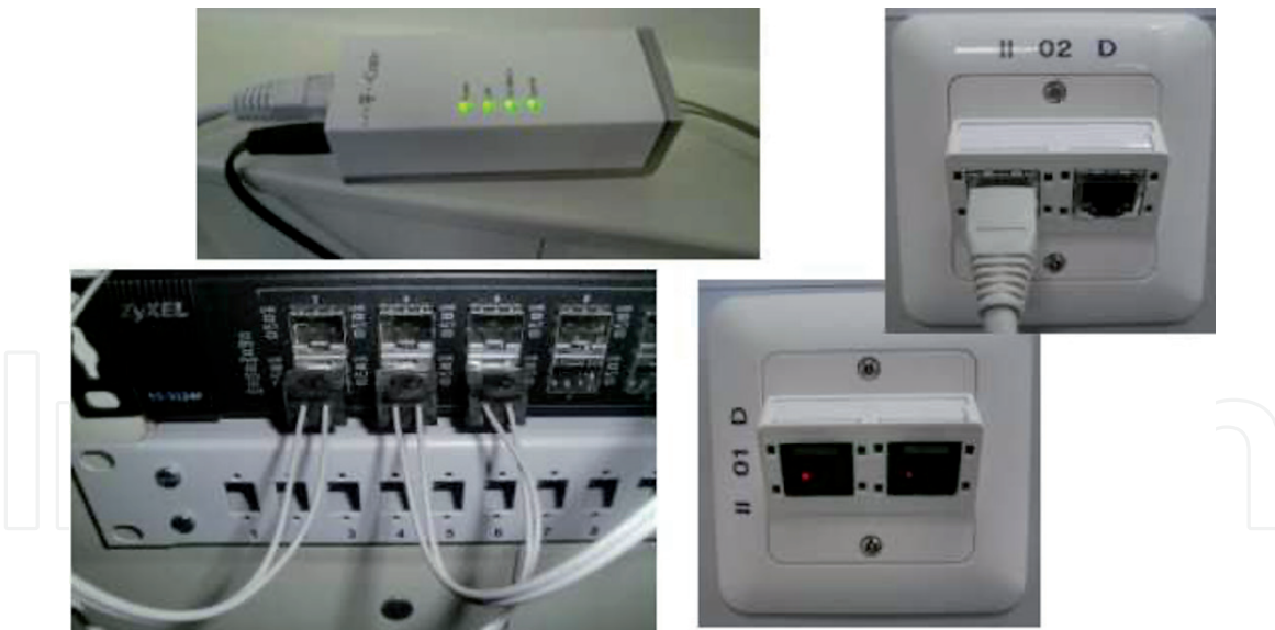
Figure 15. POF media convertors, Ethernet switches and 4-port optical POF switch RJ-45 wall outlets with WiFi-Accesspoint (Rutenbeck GmbH).
